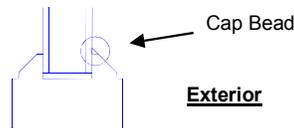
A cap-bead will further minimize the chance of water infiltration and weathering caused by exposure to precipitation.
