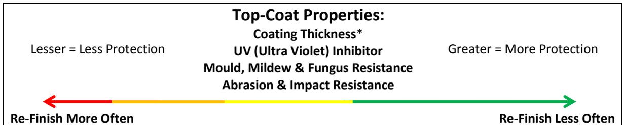
\*It is not recommended to exceed paint manufacturers maximum specified coating thickness
